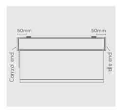
Open System Top Fix Bracket release lip must face the back of the blind.
