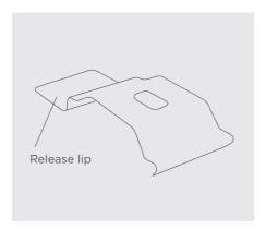
CHILDREN CAN STRANGLE IF A SAFETY DEVICE IS NOT INSTALLED. ALWAYS USE A SAFETY DEVICE TO KEEP CORDS AND CHAINS OUT OF REACH OF CHILDREN. Mark the hole positions before drilling and plugging if necessary. Use two screws in each bracket ensuring that the brackets are level. Remember to allow room for the blind to clear any obstacles when deployed, e.g. door or window handles.
